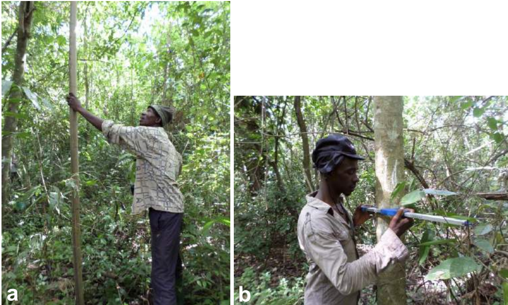
Figure 4. a) Height estimations using a Raphia pole, b) DHB measurements using a calliper.
