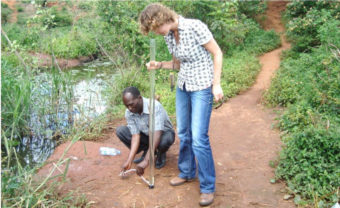
Figure 4. Using the water turbidity tube
